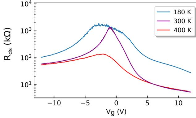
FIG. 3: Transfer characteristics of a PdSe<sub>2</sub> FET with intermediate thickness (S12bis, 28nm) at various temperatures.
