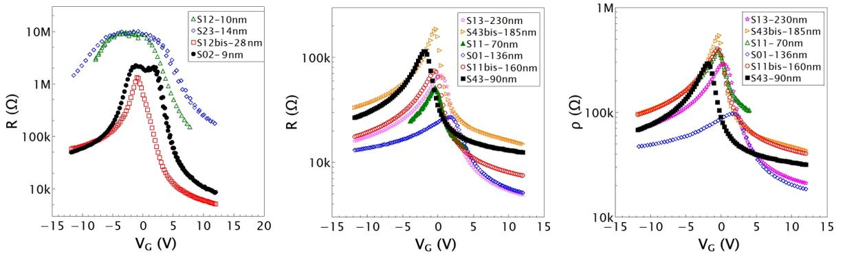
FIG. 2: Room temperature transfer characteristics of PdSe<sub>2</sub> transistors. Panel (a) corresponds to the thin-channel transistors, referred to as PdSe<sub>2</sub> 2D-FETs in the main text; Panel (b) corresponds to thick-channel transistors, referred to as PdSe<sub>2</sub>-MOSFETs in the main text. Panel (c) is a replot of Panel (b) data in terms of in plane square resistance. Representative Samples S43 and S02, detailed in the main text, are highlighted as filled black symbols.
