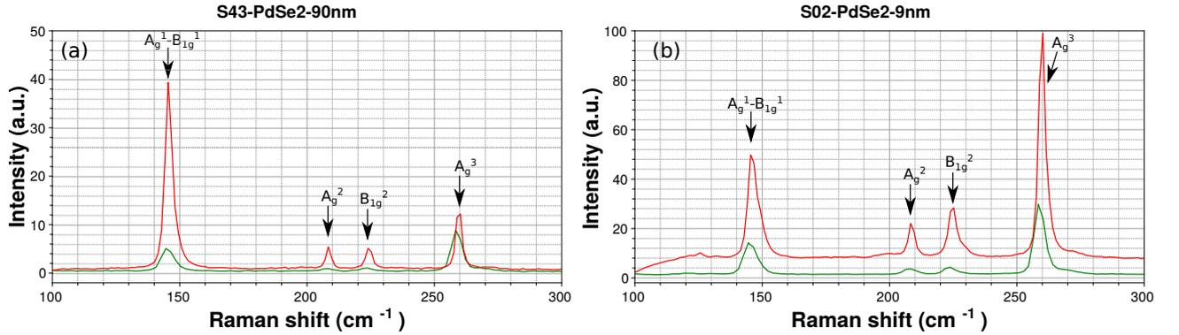
FIG. 1: Raman spectra of the thick PdSe<sub>2</sub> transistor (panel (a)) and thin PdSe<sub>2</sub> transistor (panel (b)), for a 633nm excitation line (red line) and a 532nm excitation line (green line). The Raman peaks are labeled by the corresponding Raman-active vibrational modes.
