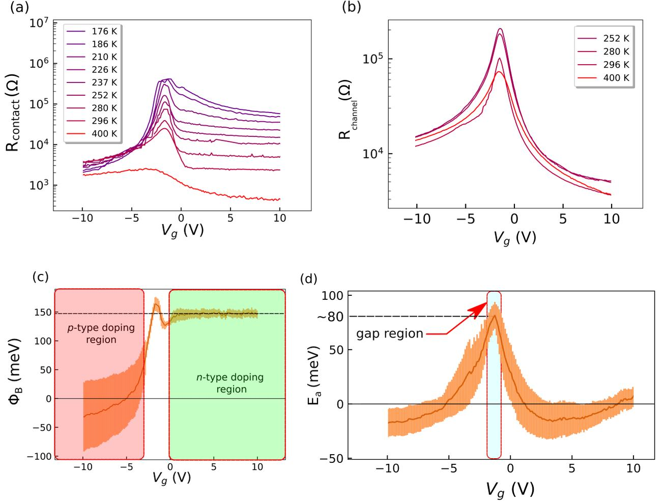
FIG. 4: Schottky barrier height and channel resistance analyses of RF admittance spectra. Deembedded contact resistance (a) and channel resistance (b) from the modeling of RF admittance spectra at various temperatures. (c) Extracted Schottky barrier height from the temperature behavior of Schottky barrier resistance (panel (a)). (d) Extracted activation energy from the temperature behavior of the channel resistance in panel (b).
