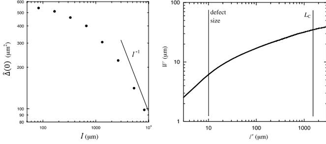
Fig. 3: Left: scaling of the correlator  $\hat{\Delta}(0) := \langle \bar{h}_l(w) \bar{h}_l(w) \rangle$  as a function of the averaging length  $l$  along the CL (here iso/Si). The asymptotic scaling  $l^{-1}$  is marginally reached for  $l = L_c$ . Right: roughness  $W(l')$  of the contact line for iso/Si. Due to the limited range between the defect size and the capillary length, no scaling is achieved.
