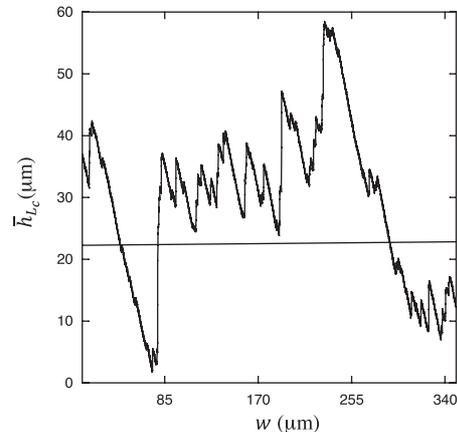
Fig. 2: Height of the contact line  $\bar{h}_{2L_c}(w)$  averaged over  $2L_c$ , as a function of the position  $w$  of the plate (system: iso/Si). The fast depinning events (upwards) are clearly visible. Between them, the CL is advected downwards at the plate velocity  $v$  (here  $1 \mu\text{m/s}$ ). The straight line is the reference level  $h_0$ .
