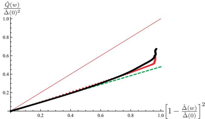
Fig. 7: (Colour on-line) Dimensionless parametric plot of  $\hat{Q}(w)/\hat{\Delta}(0)^2$  vs.  $[1 - \frac{\hat{\Delta}(w)}{\hat{\Delta}(0)}]^2$  for both experiments H<sub>2</sub>/Cs (thick red line) and iso/Si at  $v = 10 \mu\text{m/s}$  (thick black line). The thin red line is the mean-field prediction. The thick dashed green line is an extrapolation based on a loop expansion, as discussed in the text.
