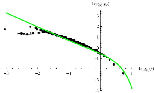
Fig. 8: (Colour on-line) The measured dimensionless avalanche-size distribution function  $p(s)$ , as defined in the text, for iso/Si. For comparison an analytical estimate, defined in eq. (11), based on a one-loop calculation with the scaled elastic kernel  $\tilde{\epsilon}_{\pi/2}(x)$ . The small-size cutoff is  $\log_{10}(s) = -2$ , *i.e.* the size of a defect.
