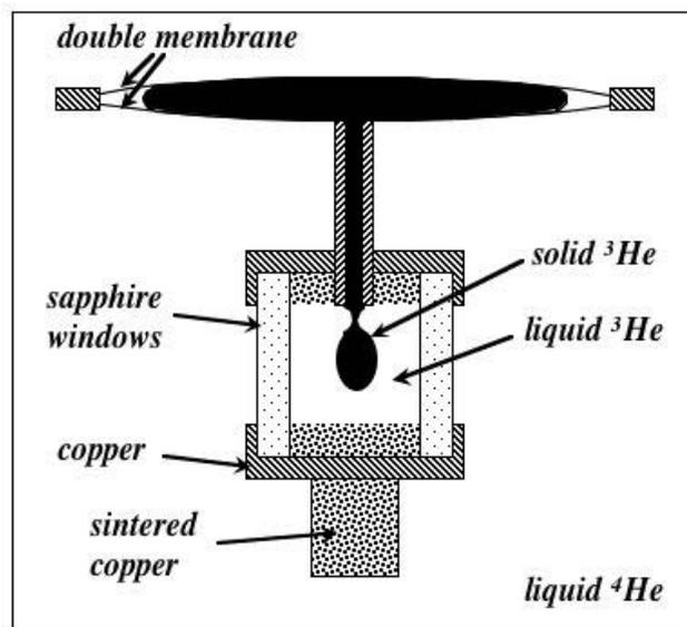
FIG. 1. The experimental cell where  $^3\text{He}$  crystals were grown thanks to a flexible membrane. The lower part was 3.45 mm wide and 3.27 mm high; it could be observed through windows from the outside of the cryostat, as shown in Fig. 2.
