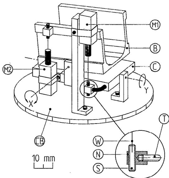
FIG. 1. Schematic view of the experimental setup: *M1* fixed motor, *M2* mobile motor, *B* boat containing the crystal, *C* cradle supporting the articulated boat, and the mobile motor *W* tungsten wire, *S* brass screw 1.5×30/100 mm, *N* stainless-steel nut, *T* nut axis (brass screw 1.5×30/100), *CB* bottom of the experimental pressurized cell.
