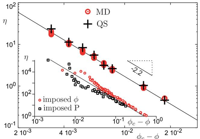
FIG. 1. Viscosity  $\eta$  as a function of volume fraction  $\phi$  measured from molecular dynamics (MD) and quasi static simulations (QS). Inset: compilation of experimental data available in the literature at imposed pressure  $P$  (with  $\phi_c = 0.587$ ) and imposed volume fraction  $\phi$  (with  $\phi_c = 0.615$ ).
