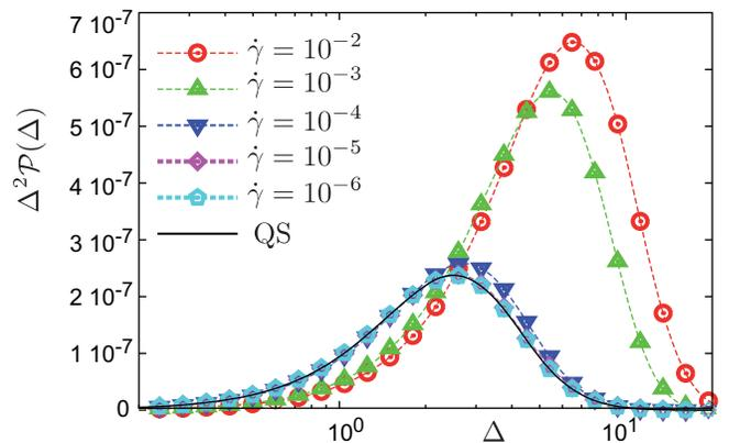
FIG. 3. Probability distribution function  $P(\Delta)$  of the rescaled velocity fluctuations  $\Delta = \delta v / \dot{\gamma}$ . It is determined from the Van Hove function measured for  $\gamma = 5 \cdot 10^{-4} = 10 \gamma_0$ , for  $\zeta = 10^{-2}$  and different strain-rates. Volume fraction  $\phi = 0.825$ .
