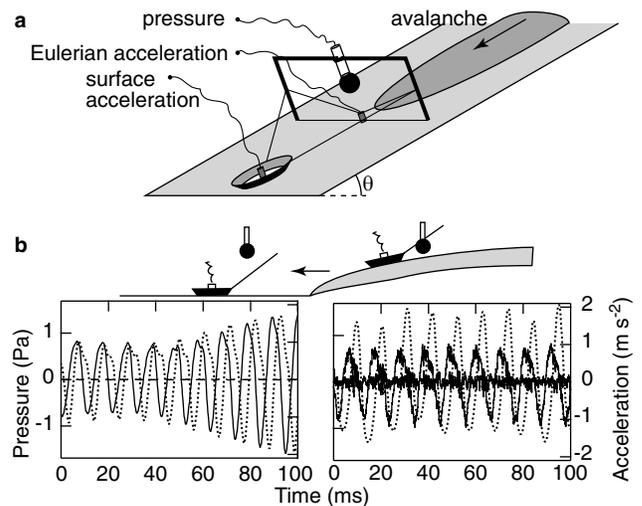
FIG. 1. (a) Measurement setup. (b) Samples of the sound (dotted line) and surface acceleration (solid line) signals, just before the avalanche front reaches the transducers (left) and just after (right). The dashed line is the same acceleration signal from which the Fourier components smaller than 500 Hz have been removed. It evidences the high frequency noise induced by avalanching grains (right), not present before the avalanche (left). The sound may be listened to at Ref. [1].
