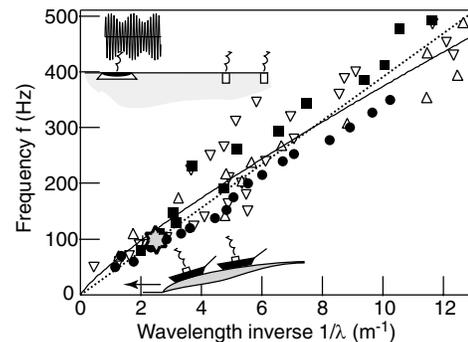
FIG. 3. Dispersion relation of surface elastic waves, the sand being at rest [transducers distant by 5 cm (down triangle), 15 cm (up triangle), 25 cm (square), and 42 cm (circle)] or avalanching (star). The dotted line corresponds to a nondispersive relation  $f = c \lambda^{-1}$ , with  $c = 40 \text{ m s}^{-1}$  and the solid line to the Rayleigh-Hertz relation  $f = c_0^{2/3} g^{1/6} \lambda^{-5/6}$ , with  $c_0 = 230 \text{ m s}^{-1}$ .
