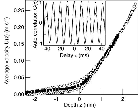
FIG. 4. Average velocity profile in a laboratory avalanche for different flow heights:  $H = 8d$  (triangle),  $H = 10d$  (square),  $H = 15d$  (circle). The solid line corresponds to the velocity profile  $U(z) = fz$  with the sound frequency  $f = 100 \text{ Hz}$ . Inset: Autocorrelation of the microphone signal measured in the core of a steady and homogeneous avalanche (solid line) and a very intermittent one (dotted line).
