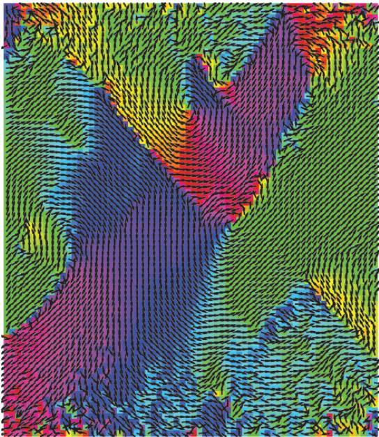
We have recently shown that a model knitted fabric exhibits crackling noise in its force response that corresponds to extended fault-like slip bands in its spatial deformation field. The scale invariance displayed by these features, together with their morphology, is strongly reminiscent of seismic events. This system can thus, to some extent, be considered as a toy model for earthquakes.
