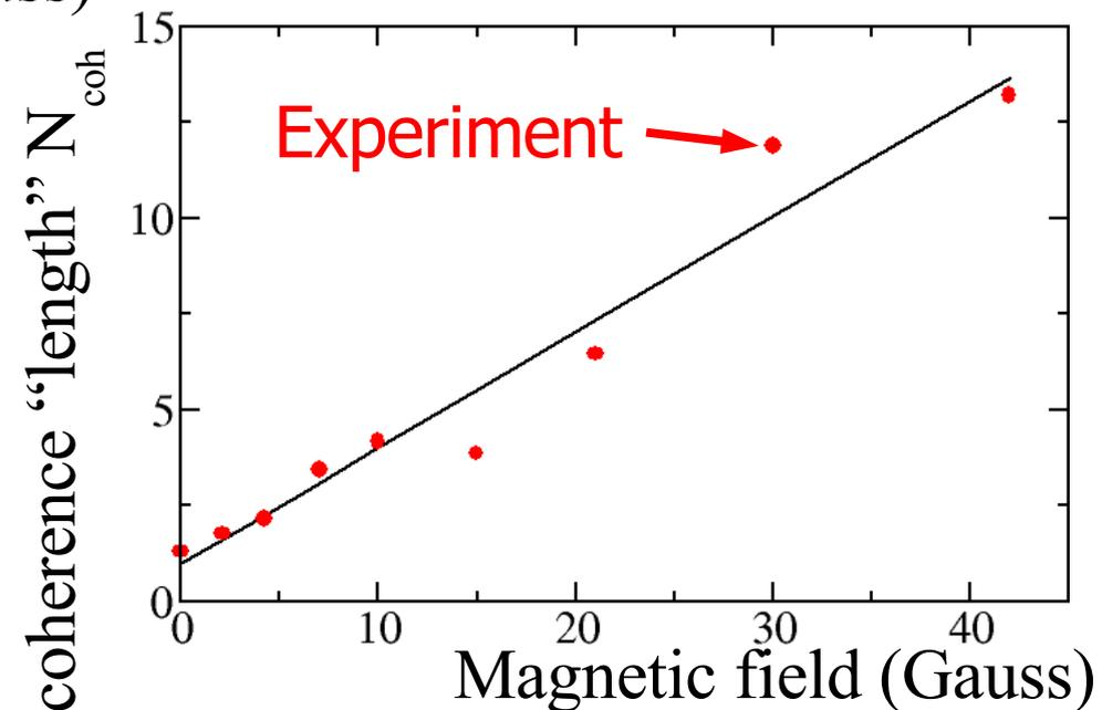
Full contrast of the CBS interference is restored at large magnetic field
