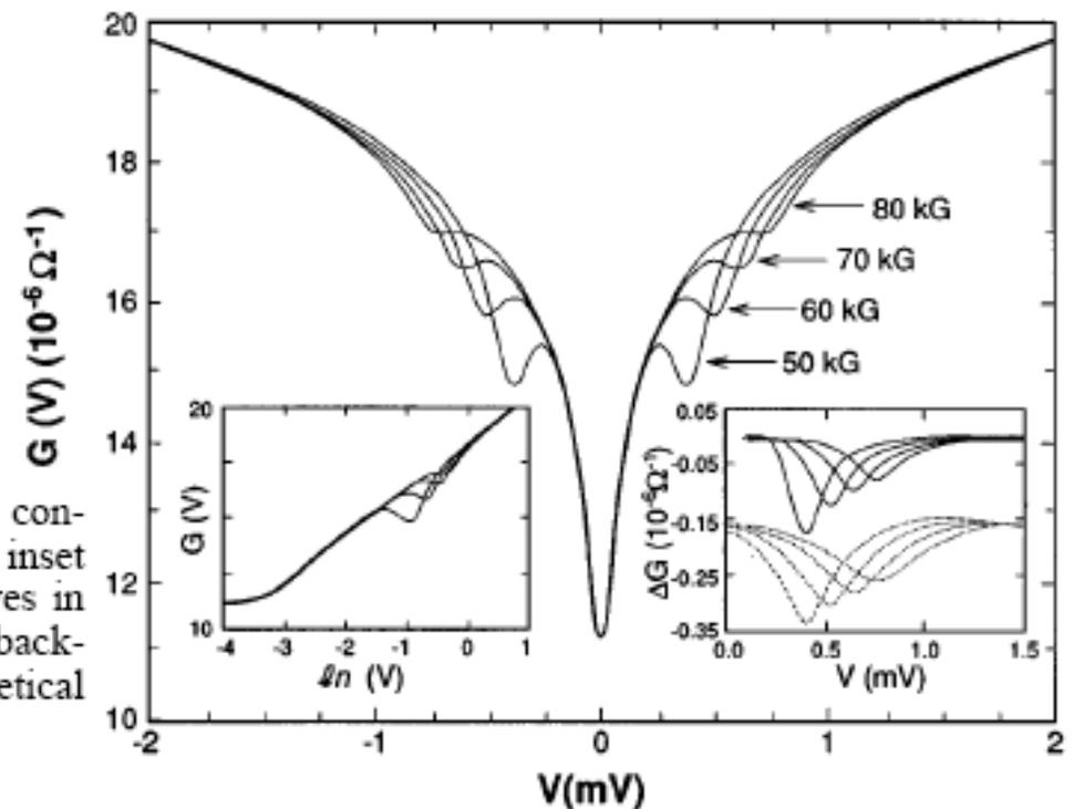
FIG. 2. The main figure is the normal state tunneling conductance of the film in Fig. 1 at several  $H_{\parallel}$ . The left inset shows the  $\ln(V)$  dependence of the ZBA. The solid curves in the right inset show the Zeeman anomaly with the  $\ln(V)$  background subtracted off. The dashed curves are the theoretical DOS of Ref. [3] and have been shifted down for clarity.
