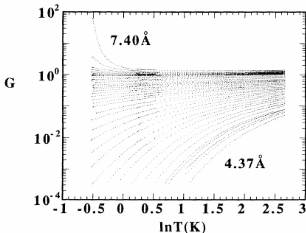
FIG. 1. Logarithm of the conductance  $G$ , in units of  $4e^2/h$ , vs  $\ln(T)$  for a number of different Bi films. The thickness of the first (thinnest) and last (thickest) films are indicated.
