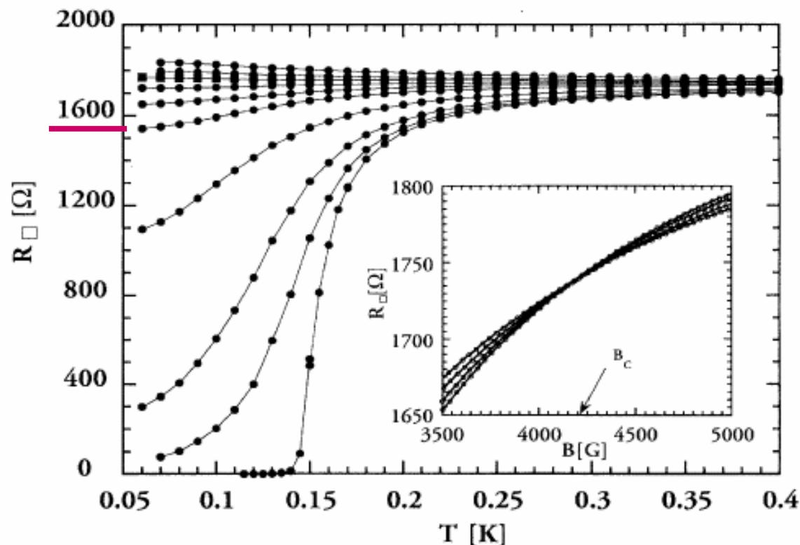
FIG. 1. Zero bias resistance of sample 2 plotted versus temperature at  $B = 0, 0.5, 1.0, 2.0, 3.0, 4.0, 4.4, 4.5, 5.5, 6$  kG. In the inset,  $R_{\square}(B, T, E = 0)$  for the same sample measured versus field, at  $T = 80, 90, 100, 110$  mK.
