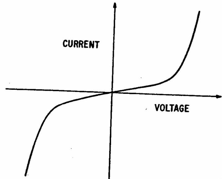
Fig. 1. Schematic drawing of a tunneling experiment. If the capacitor plates are spaced about  $50 \text{ \AA}$  apart or less, a tunnel current will be easily observable. The current-voltage characteristic will be nearly symmetric about zero, linear at low voltages (below  $\sim 0.1 \text{ V}$ ), and nonlinear at higher voltages.
