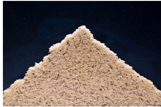
Figure 58. Stable configuration in a rice pile experiment. (Photo by the author.) The grains are between two glass plates 5 mm apart. The pile was prepared by slowly increasing the inclination of the plates from horizontal to vertical. Brighter grains sit at the top and are more likely to topple.
