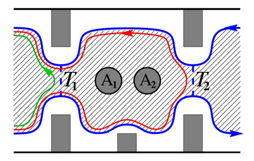
$$\sigma_{xx} \propto |t_1|^2 + |t_2|^2 + 2|t_1t_2| M_{bc} |\cos(\beta + \theta_{bc})$$
