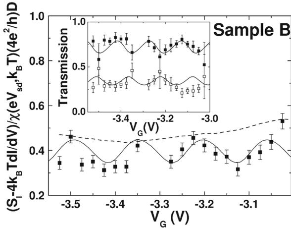
FIG. 5. Noise power spectral density measured (closed squares) at  $V_{SD} = -0.7$  mV normalized by  $\chi(eV_{sd}, k_B T) \times 4e^2/h \times D$  as a function of  $V_G$  for sample B. The Johnson-Nyquist noise  $4k_B T dl/dV$  has been subtracted to allow a direct determination of  $D_1$  and  $D_2$ . The dashed lines correspond to the theory with the assumption of full orbital degeneracy, in clear disagreement with the noise data. Inset: Gate dependence of  $D_1$  and  $D_2$ .
