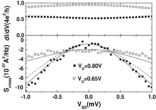
FIG. 3. Top: Nonlinear conductance as a function  $V_{SD}$  for gate voltages  $V_G = 0.65$  V and  $V_G = 0.80$  V for sample A. The closed squares correspond to  $V_G = 0.65$  V and the open squares correspond to  $V_G = 0.80$  V. Bottom: Corresponding noise power spectral density as a function  $V_{SD}$ . The lines correspond to formula (2) used for  $D = 0.542$  and  $D = 0.95$  which are the zero bias values of  $dI/dV$  for  $V_G = 0.65$  V and  $V_G = 0.80$  V in units of  $4e^2/h$ .
