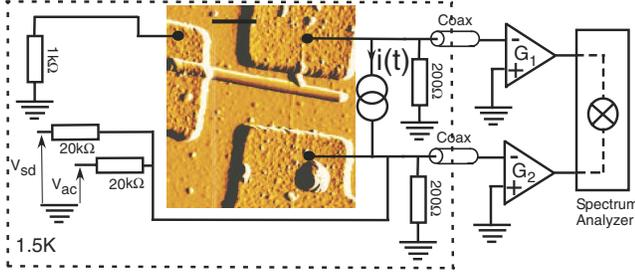
FIG. 1 (color online). Diagram of the circuit and AFM picture of one of the samples (sample A) presented in this Letter. The MWNT is shunted by a 1 k $\Omega$  resistor placed on the PCB. The bar is 500 nm.
