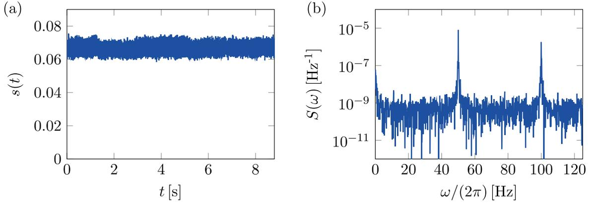
**Figure C1.** (a) Time evolution of the saturation parameter  $s$ , for the smallest mean value  $s = 0.065$  explored in figure 4(b). The rms fluctuations of  $5 \times 10^{-3}$  result from the  $\sim 80$  dB dynamic range of the intensity locking system. (b) Spectral density  $S(\omega)$  of the saturation parameter noise corresponding to (a).
