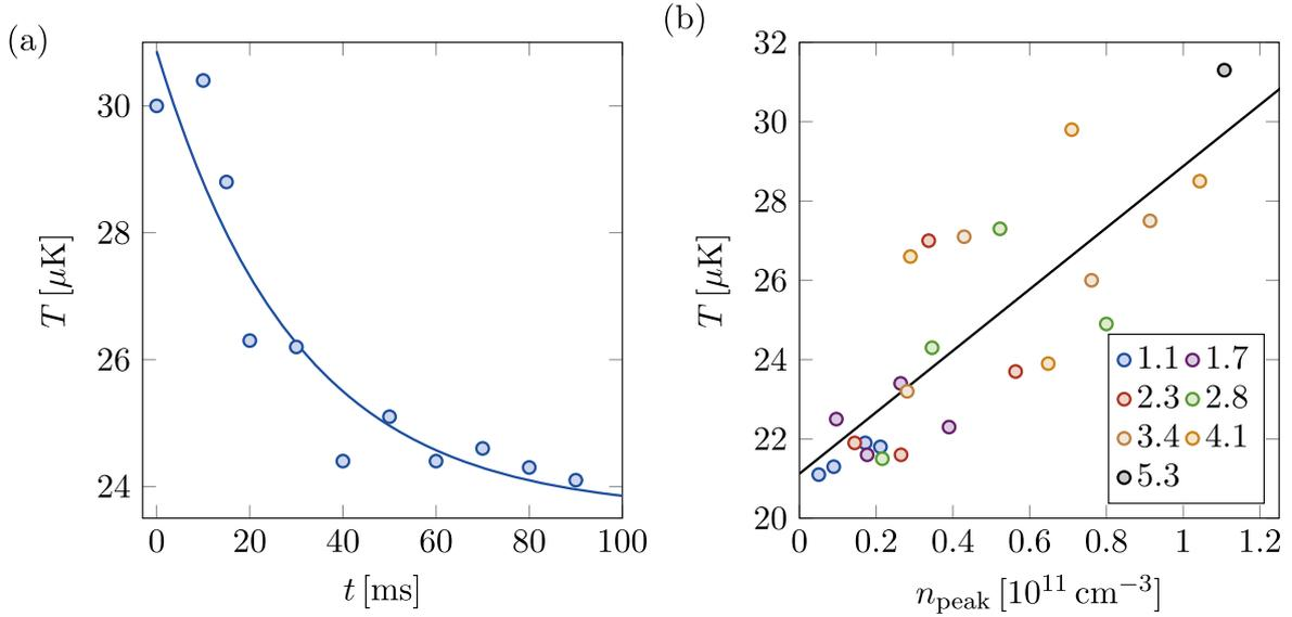
**Figure A1.** (a) Evolution of the gas temperature  $T$  with time  $t$  right after the MOT parameters are set to the ‘compressed MOT’ values. The solid line is an exponential fit of the equilibration dynamics. (b) Temperature  $T$  as a function of atom density  $n$ , measured for various atom numbers and gradient values, indicated in the legend (in  $\text{G cm}^{-1}$ ). The solid line is a linear fit of slope  $\gamma = 8(1) \times 10^{-11} \mu\text{K cm}^3$ .
