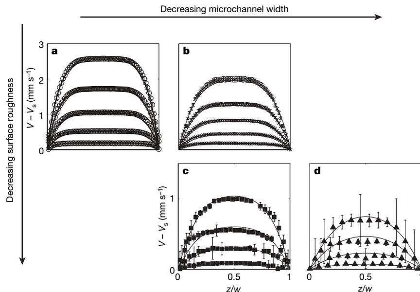
**Figure 2 | Velocity profiles in microchannels with different widths  $w$  and confining wall roughness, corrected for the slip velocity.** **a**, Rough microchannel with  $w = 250 \mu\text{m}$ ; **b**, rough microchannel with  $w = 125 \mu\text{m}$ ; **c**, smooth microchannel with  $w = 112 \mu\text{m}$ ; and **d**, smooth microchannel with  $w = 56 \mu\text{m}$ . Plotting symbols show data points; solid lines show velocity profiles predicted by the non-local model of equation (1) with a flow
