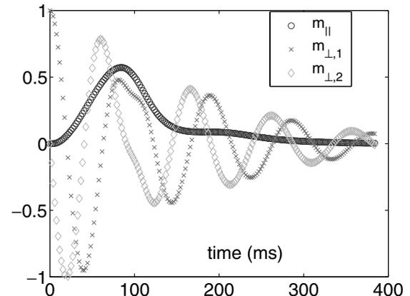
FIG. 1. Time evolution of the spin polarization  $\mathbf{m}$  at the center of the trap;  $m_{\parallel}$  corresponds to the population difference between the two states;  $m_{\perp,1}$  and  $m_{\perp,2}$  are the two components of the transverse spin polarization. The center-to-edge difference in Bohr frequency  $\delta\Omega/2\pi$  is 12 Hz.
