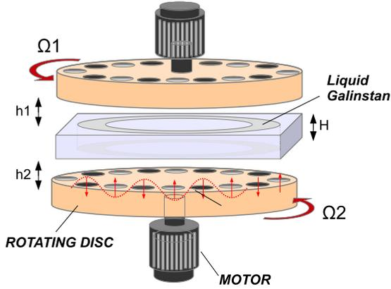
FIG. 1. Schematic view of the experiment. A flow of liquid metal (Galinstan) is driven in an annular channel by the Lorentz force due to a traveling magnetic field created by magnets placed on rotating disks.
