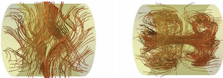
Fig. 2. Numerical simulations of the magnetic field at dynamo threshold: left: an equatorial dipole is obtained when only the mean flow is taken into account. Right: an axial dipole is generated when non axisymmetric components in the form of vortices generated by the blades are included in the velocity field.
