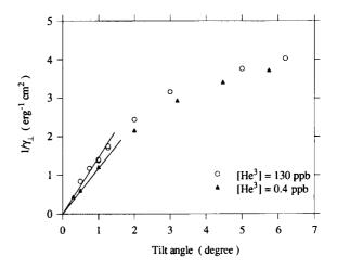
Fig. 1. Measurements of the component  $\gamma_{\perp}$  of the surface stiffness as a function of the orientation at T = 0.2 K. The circles correspond to regular helium 4 ([<sup>3</sup>He] = 130 ppb), and the triangles to ultrapure helium 4 ([<sup>3</sup>He] = 0.4 ppb).
