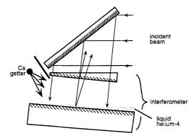
Fig. 1. Schematic drawing of the experimetal setup. The diameter of the mirror is 30 mm and the spacing between the mirror and the semi-reflecting plate is 10 mm.
