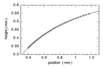
Fig. 3. Experimental profile of an advancing meniscus (dots) at 0.83 K, and theoretical profile (full line). The only adjustable parameter is the position of the contact line. The contact angle  $\theta_a$  is found equal to 25.5  $\pm$  0.5 °.
