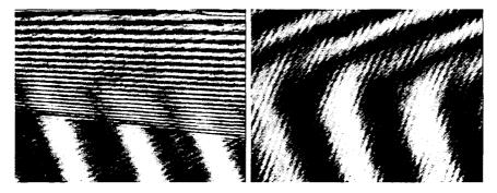
Fig. 2. Interferometric images of an advancing meniscus (left) below the wetting temperature (T = 0.83 K) and (right) above the wetting temperature (T = 1.95 K). The part of the mirror covered by the liquid wedge is the upper part of the images. The actual size of the images is  $1.85 \times 1.39$  mm.
