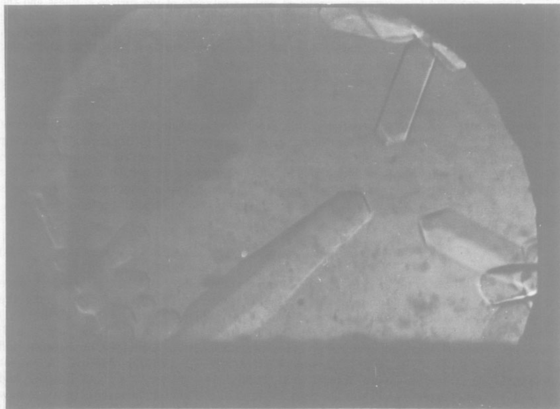
Fig. 1. — ^3\text{He} crystals growing slowly at 70 mK ( T < T_R , v < 1 \mu\text{m}/\text{s} ). The facets of the polyhedrons are 110 facets.
