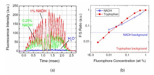
Fig. 3. Optical filter-based system response to fluorophore-doped water droplets. (a) Real-time fluorescence channel recordings for single NADH particles (with two non-functioning 340nm LED array elements after the 1 msec mark) shown for two concentration levels measured against pure  $H_2O$ , and (b) the measured fluorescence to scatter ratios for both the 290nm array targeting tryptophan (closed circles) and the 340nm array targeting NADH (open circles).
