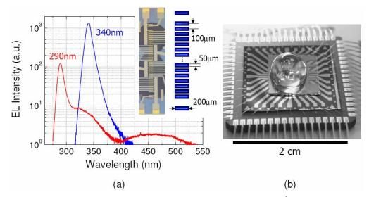
Fig. 1. (a) Electroluminescence spectra on a semi-log scale taken under 1 kA/cm<sup>2</sup> injection current from typical elements of a 290 nm and 340 nm linear array. Light output axes scaled and not comparable for different devices. Inset shows array geometry and individual LED element dimensions. (b) Photographic image of packaged array.
