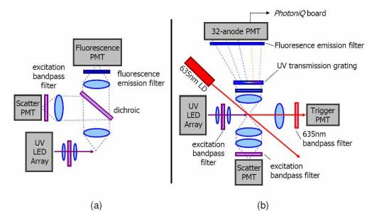
Fig. 2. Top-view schematics of two compact LED array-based detection systems. (a) Optical filter-based and (b) spectroscopic fluorescence detection.
