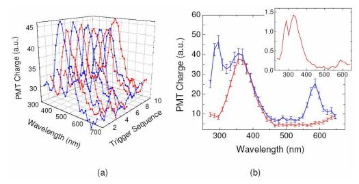
Fig. 4. Single particle fluorescence spectra. (a) Ten sequential 0.025% NADH-doped water droplets under 340 nm excitation. (b) 290 nm excitation of single 0.5% tryptophan-doped water droplets with (lower curve) and without (upper curve) an additional LED-scatter blocking filter. Inset shows average over 500 particles of  $6 \,\mu$ m diameter dry tryptophan.
