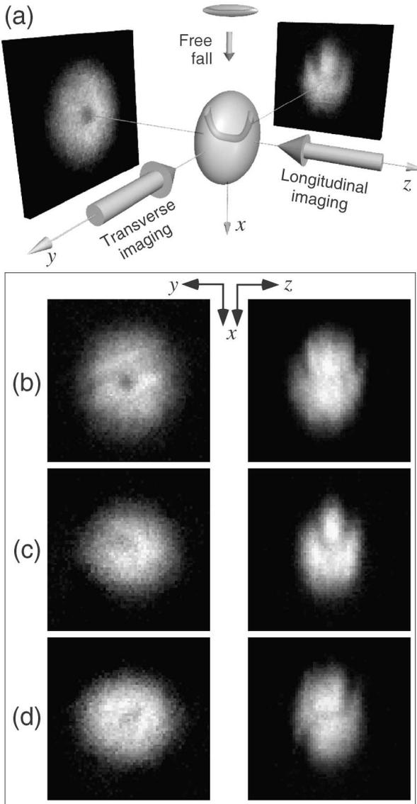
FIG. 1. (a) Schematic of the imaging system. The cigar shaped condensate is imaged after 25 ms of time of flight leading to the inversion of the ellipticity in the  $xz$  plane. Two beams image the atom cloud simultaneously along the longitudinal ( $z$ ) and transverse ( $y$ ) directions of the initial cigar. (b)–(d) Simultaneous longitudinal and transverse images of condensates after  $\tau = 4$  s (b),  $\tau = 7.5$  s (c), and  $\tau = 5$  s (d).
