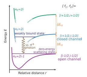
FIG. 1. (Color online) Fano-Feshbach resonance in a collision between two atoms, induced by an oscillatory magnetic field. If the mw frequency  $\omega$  approaches the energy difference between the incident scattering state and a weakly bound dimer state, the pair of atoms undergoes virtual spin-flip transitions which cause a resonant variation of the scattering length with  $\omega$ .
