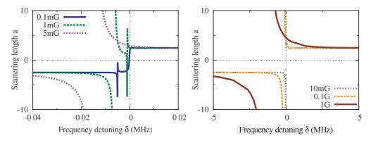
FIG. 2. (Color online) Resonance in <sup>133</sup>Cs involving the bound state with energy  $|E_T| = h5 \text{ kHz} = \mu_B 4 \text{ mG}$ , for  $B_0$  ranging from 0.1 mG to 1 G, calculated using method (ii). The scattering length *a* is expressed in units of 1000  $a_0$ .
