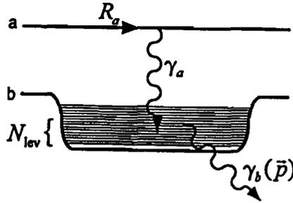
Figure 1: A model for an atom laser: atoms are injected with rate  $R_a$  in internal state  $a$ . They decay to the internal state  $b$ , and are then trapped inside a box of volume  $V$ . The laser action originates from the stimulated emission of atoms in states  $|b, \vec{p}\rangle$  when these states are already occupied.
