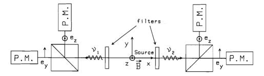
Fig. 3. Experimental scheme. The photomultipliers detect the fluorescence photons with polarizations  $e_y$  and  $e_z$ , and the four corresponding time-delayed coincidence spectra are monitored simultaneously.
