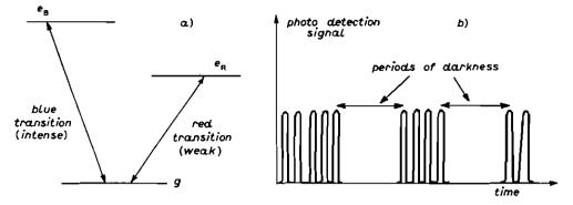
Fig. 1. -a) 3-level atom with two transitions starting from the gound state g. b) Random sequence of pulses given by a photodetector recording the fluorescence of a single atom. The periods of darkness correspond to the shelving of the electron on the metastable level  $e_{\rm R}$ .
