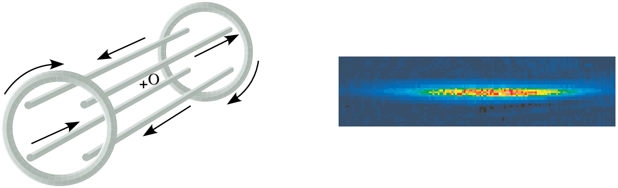
FIGURE 7: Magnetic trapping of neutral atoms. Left: Ioffe-Pritchard trap, consisting in 4 linear conductors and two circular coils. The arrows indicate the current direction in each conductor. The modulus of the magnetic field has a non zero local minimum at the center of symmetry O of the system. Atoms with a magnetic moment antiparallel to the local magnetic field are confined around O . Right: photograph of 10^7 cesium atoms confined in a Ioffe-Pritchard trap. The image of the cigar-shaped atom cloud has been obtained by recording the absorption of a short resonant laser pulse and making the image of the shadow of the atom cloud onto a CCD camera. The temperature is of the order of 10 microkelvins (photograph: ENS).
