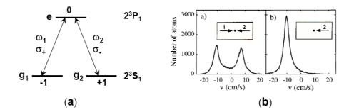
Figure 4: VSCPT experiment. (a): three Zeeman sublevels involved in the VSCPT cooling experiment described in this section. (b): the left part shows the double peak velocity distribution obtained in this experiment. The fact that the two peaks are resolved proves the subrecoil character of the cooling. The right part of the figure shows that a single peak without any loss of atoms is obtained when one of the 2 lasers is switched off slowly.
