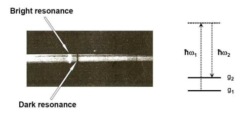
Figure 1: Bright and dark resonances observed in the fluorescence light emitted by a sodium vapor put in a spatially inhomogeneous magnetic field. The dark resonance appears at a point where the frequency difference  $\omega_1 - \omega_2$  between two laser modes matches the frequency splitting between two Zeeman sublevels  $g_1$  and  $g_2$ .
