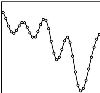
Figure 2.5: Rugged energy “landscape” which poses problems in a dynamical Monte Carlo simulation at low temperatures. The system will be stuck in one of the local minima, and the dynamics will be futile, i. e. very repetitive.
