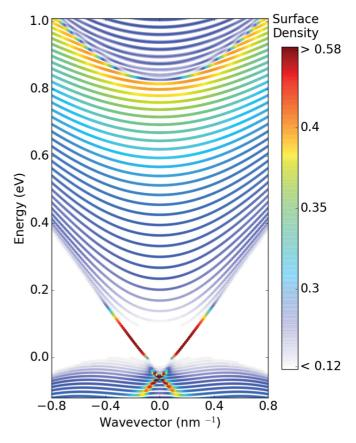
FIG. 8. Numerical dispersion relation  $E(k_{\parallel})$  for an HgTe/CdTe interface obtained within a six-band Kane model.  $k_{\parallel}$  corresponds to the momentum along the interface. The color encodes the density of eigenstates in a region of ~6 nm around the interface. The existence of localized states around the interface is shown within the gap but also at high energy around 1 eV.
