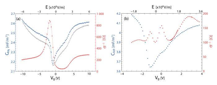
FIG. 5. High electric-field capacitance and resistivity measurements in samples (a)  $S_A$  and (b)  $S_B$ . The low-frequency data [gray dots in (a)] are added for comparison. To overcome hysteresis, the data are plotted for an increasing gate voltage. The most prominent features are the apparition of additional resistance peaks in the electron regime, with the Dirac peak being signaled by the capacitance dip. In sample  $S_A$ , the resistance peak is accompanied by a bump in the capacitance.
