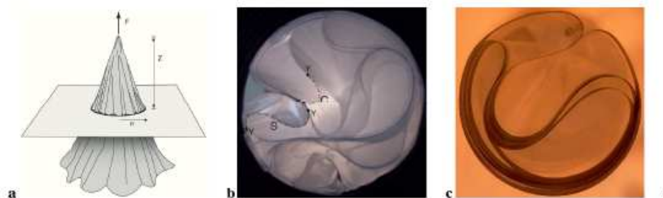
Fig. 5.1: (a) A schematic setup for conical packing. (b) Typical pattern at high confinement. The different curves appearing during the "growth of the elastic rod" are also depicted. (c) A typical pattern observed at lower confinement showing the emergence of complex structures [21].
